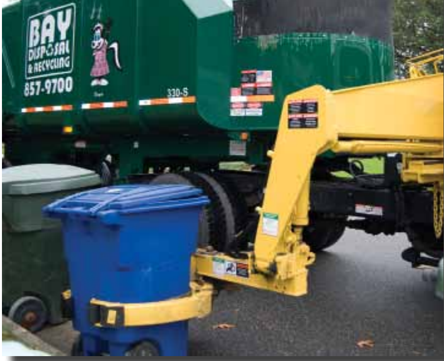
Pincers grasp a cart as Bay Disposal & Recycling collects recyclables in Newport News, VA.
