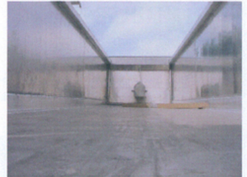
Ejector ram cylinder sized to completely unload trailer. Self-adjusting UHMW wipers on sides and bottom.
