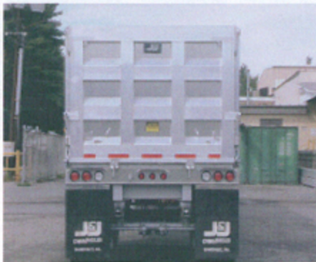
Barn door, top hinged, or hydraulic operated rear doors with full seals available.
