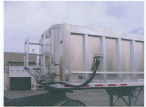
Front cow's nest with ladder optional. Controls can be mounted at top of bulkhead.
