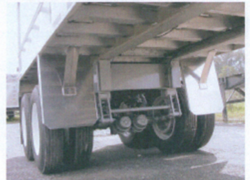
4" x 4" extruded boxed channel crossmembers. T-section longmembers running full length of trailer.
