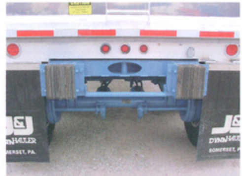
Standard bumper with extra wide blocks protects the trailer from damage due to many years of tipping.
