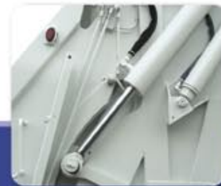
Smaller cylinders deliver more packing power and enable increased payloads.
